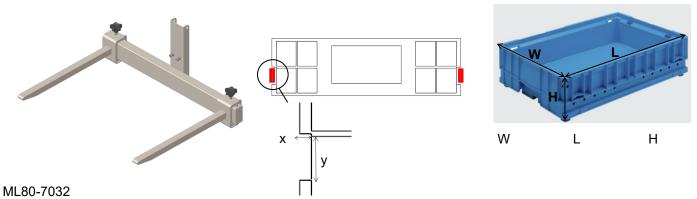
Forks with floating fingers: the forks are lowered down onto the crate and the fingers fall into spaces on the sides of the crate. To release, go down a few mm and pull the forks backwards - the round shape of the fingers float over
