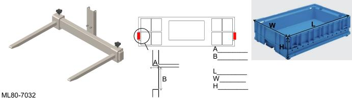
Forks with floating fingers: the forks are lowered down onto the crate and the fingers fall into spaces on the sides of the crate. To release, go down a few mm and pull the forks backwards - the round shape of the fingers float over
